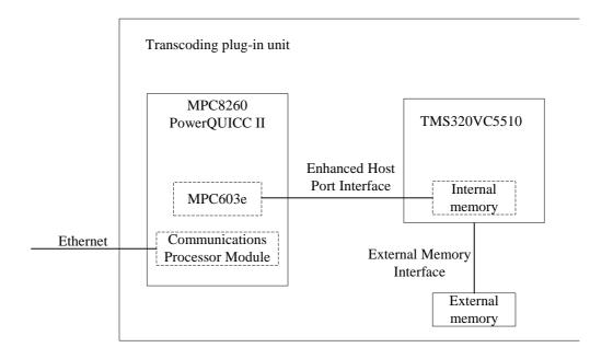
Figure 6.4 A portion of a TPU showing one host and one slave processor.
