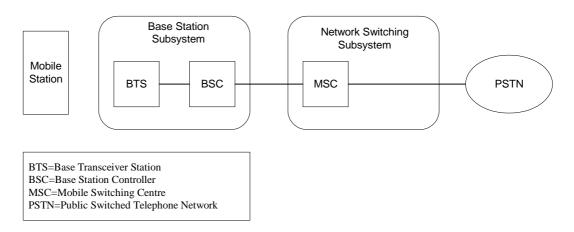
Figure 2.1 Simplified GSM architecture.
