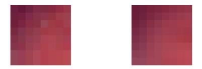
Figure 4.3 The last 8x8 block of the Lena image before and after JPEG coding.
