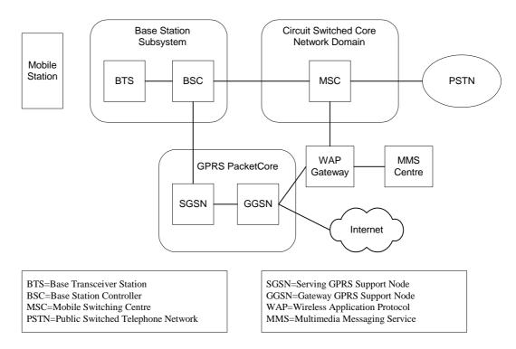
Figure 2.4 Architecture of WAP implementation of MMS.
