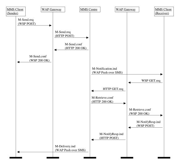
Figure 2.5 Signalling of successful sending of an MMS message.
